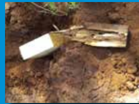
Treated and untreated wood damage
